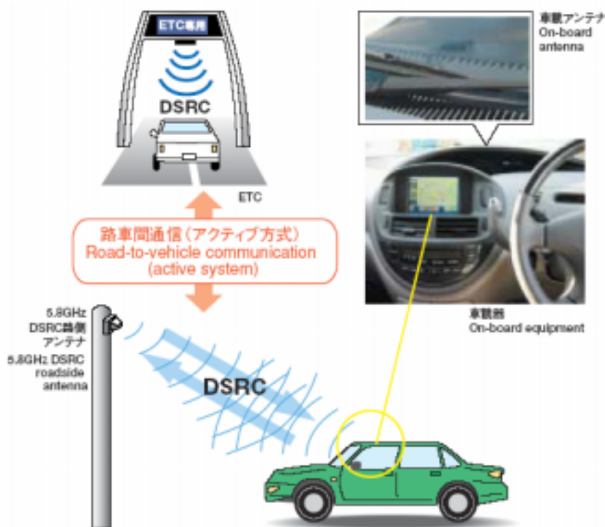
FIGURE 1. THE PRINCIPLE OF THE DSRC SYSTEM
